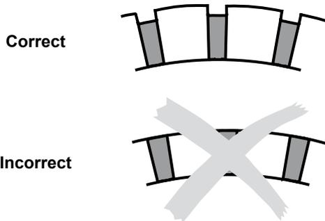
If the position has not been marked, set the brush-holder in place as follows:
